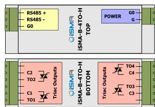
All GO terminals are connected together internally
