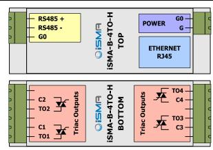
All GO terminals are connected together internally
