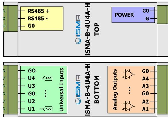
All G0 terminals are connected together internally
