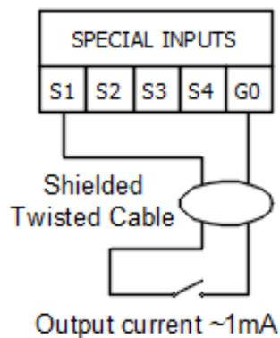
Figure 12 Connection of Special Inputs Dry Contact
