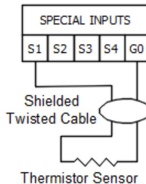
Figure 15 Connection of Special Inputs NTC sensor
