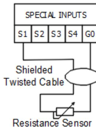
Figure 14 Connection of Special Inputs resistance sensor
