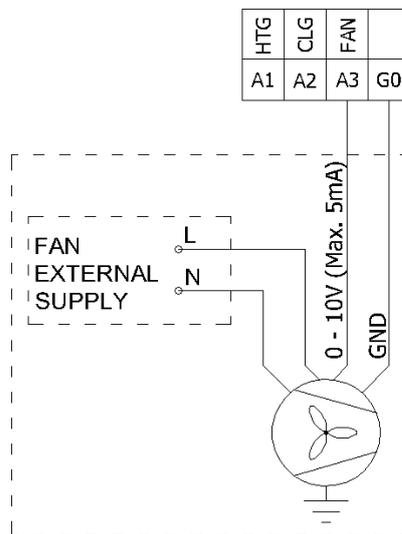
Figure 23 Analog Outputs, an exemplary connection of analog 0-10 V fan control
