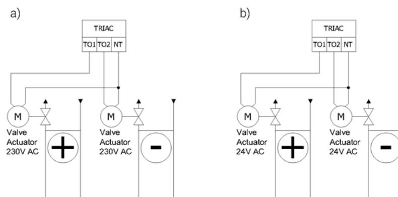
Figure 17 Connection between Thermal Valves and Triac Outputs: a) iSMA-B-FCU-HH; b) iSMA-B-FCU-HL, and iSMA-B-FCU-LL
