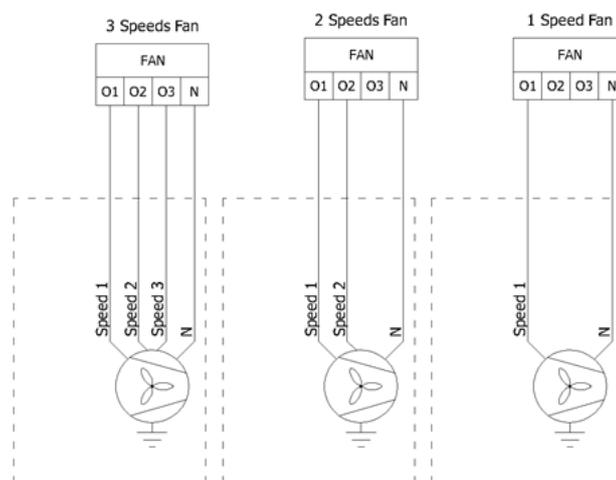
Figure 18 Digital Outputs O1-O3, example of fan connections
