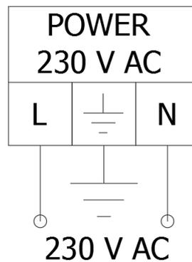
Figure 5 230 V AC Power supply connection
