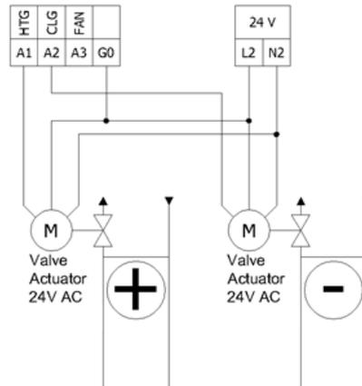
Figure 22 Analog Outputs, an exemplary connection of analog 0-10 V valve actuators
