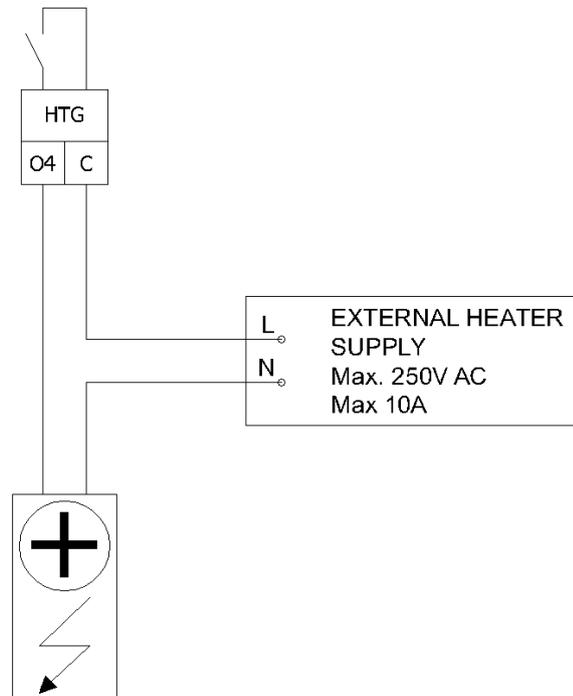
Figure 19 Digital Output O4, exemplary Electrical Heater connection
