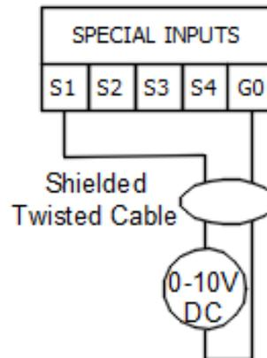
Figure 13 Connection of the Special Inputs voltage sensor
