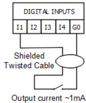
Figure 16 Connection of Digital Inputs Dry Contact
