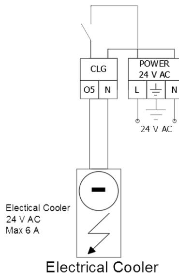
Figure 21 Digital Output O5, an example of 24 V AC Electrical Cooler connection (iSMA-B-FCU-LL version)
