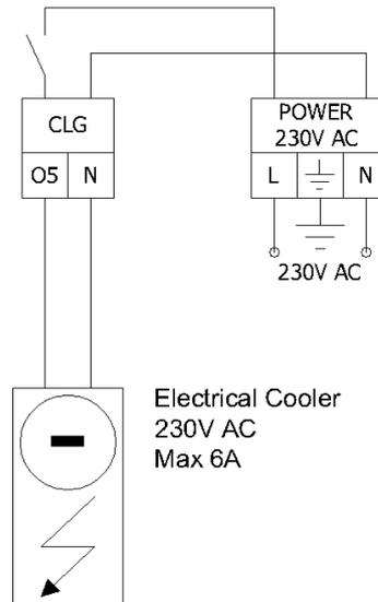
Figure 20 Digital Output O5, an example of 230 V AC Electrical Cooler connection (iSMA-B-FCU-HH and iSMA-B-FCU-HL version)
