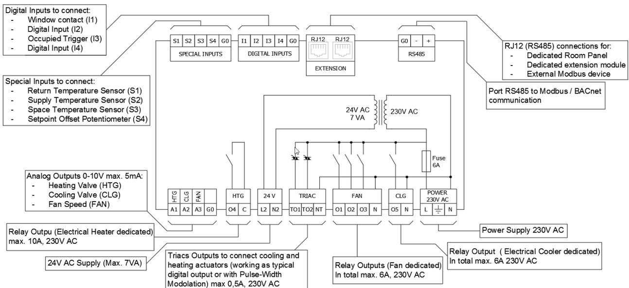
Figure 2 iSMA-B-FCU-HH diagram of terminals and internal connections
