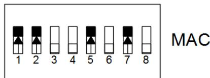
Figure 10 MAC DIP switch address 83 settings
