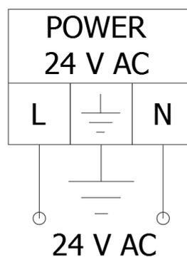
Figure 6 24 V AC Power supply connection
