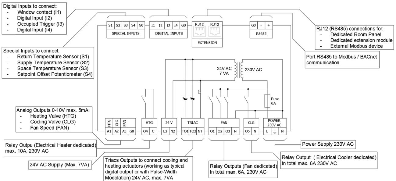
Figure 3 iSMA-B-FCU-HL diagram of terminals and internal connections
