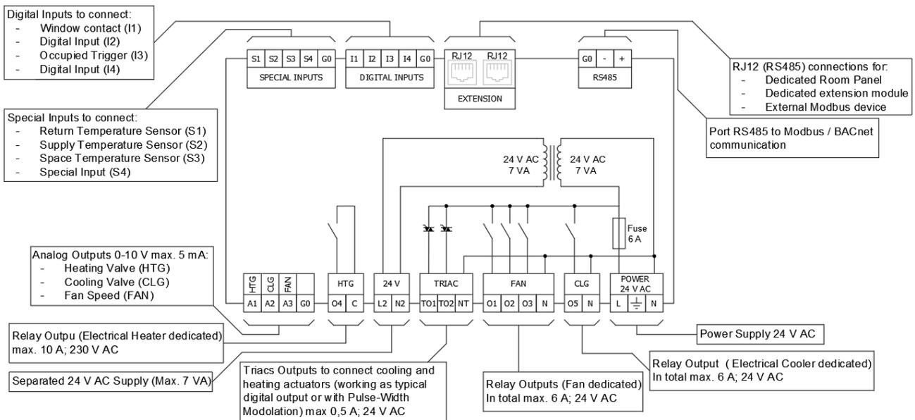
Figure 4 iSMA-B-FCU-LL diagram of terminals and internal connections
