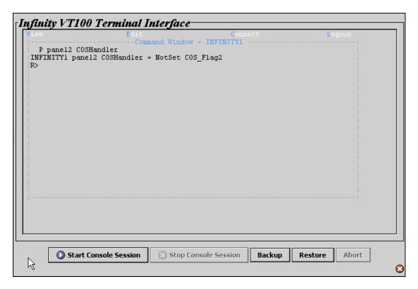
The Infinity VT100 Terminal Interface view shows the VT100 interface of the Infinity device to which driver is connected. It shows the real-time communications that are taking place from the controller to the panel.
