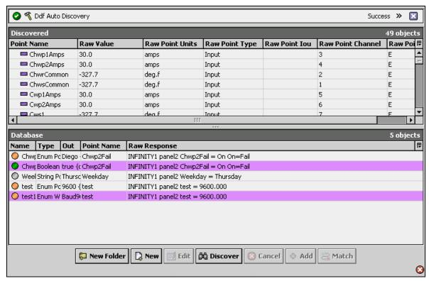
The display line for a learned point shows the point name and several columns that are the information returned from the "View/Points" and/or the "View/System Variables" menus of the Infinity VT100 interface. The "raw" columns are displayed to assist the integrator in selecting the proper points to be added to the database – the "raw" columns are not retained as properties of the point after it is added to the database.
