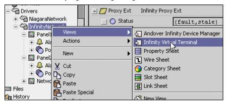
The virtual terminal view allows the user to monitor the driver activity as it is happening in real time. In addition, the user can interrupt the normal driver communications to perform interactive VT100 commands with the Infinity system, or to perform backups and restores of the system:
