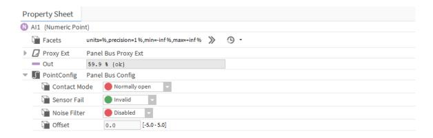
Figure 4: Panel Bus point config
