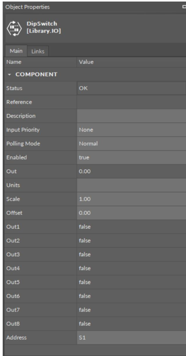
Figure 191. The DipSwitch component slots
