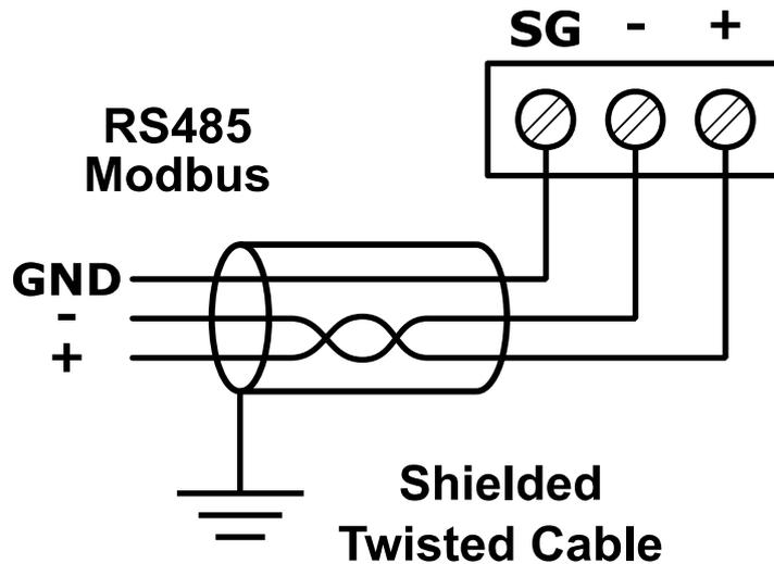
Figure 5. RS485 communication bus connection
