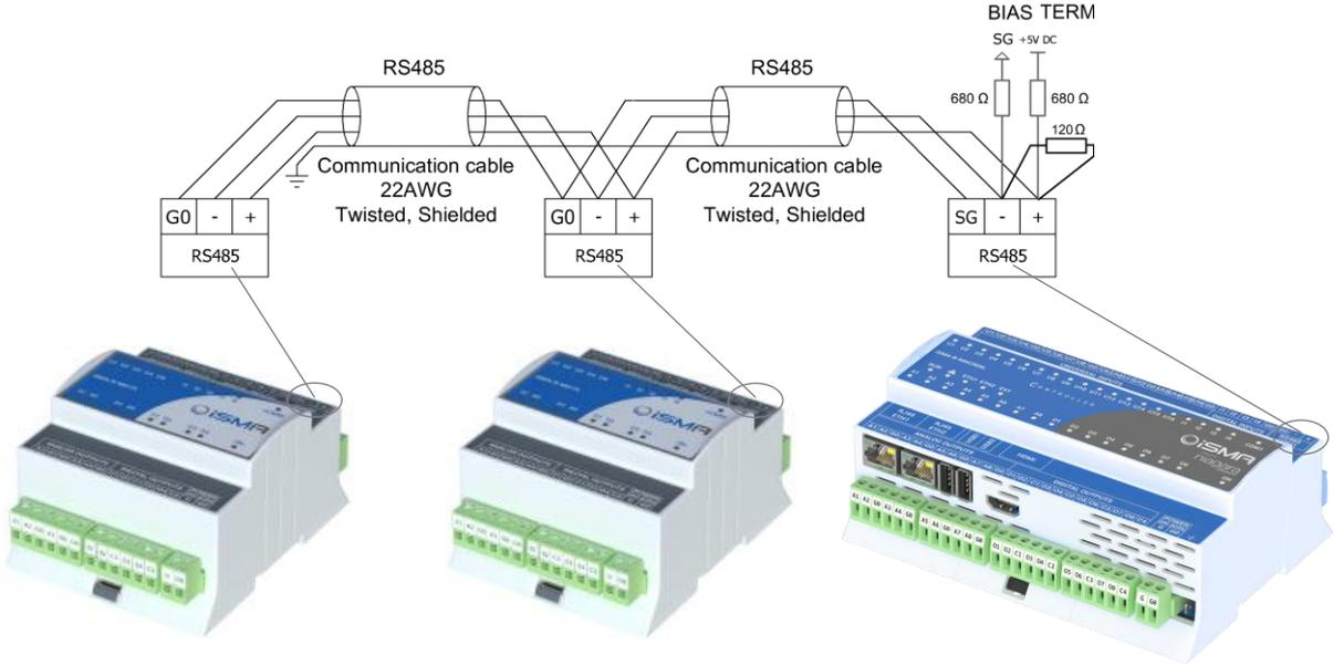
Figure 7. RS485 network termination and biasing
