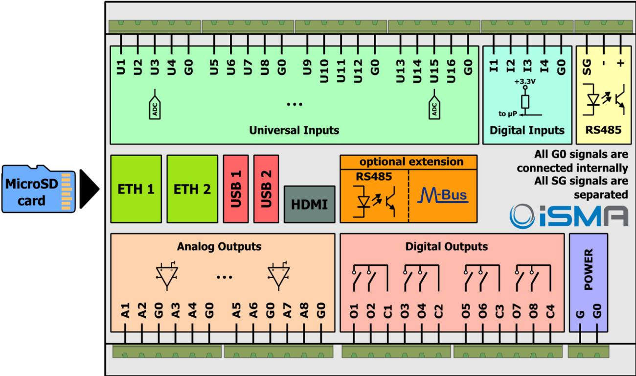
Figure 3. iSMA-B-MAC36NL Block Diagram
