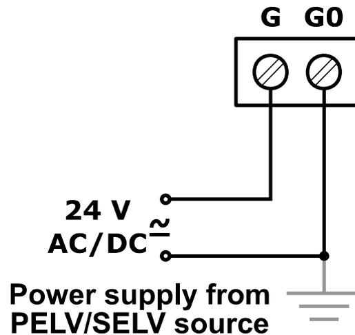
Figure 4. 24 V AC/DC power supply connection
