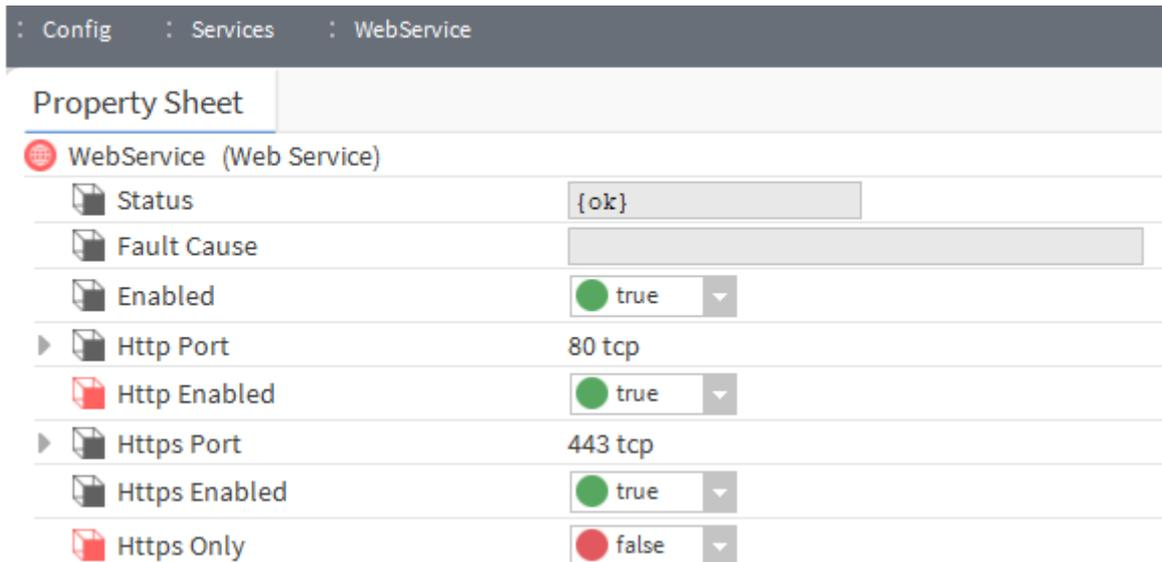
Figure 40. Proper WebService configuration for HDMI support
