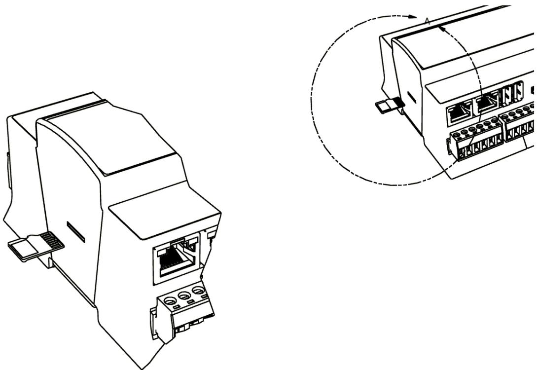
*Figure 12. SD Card Mounting*
