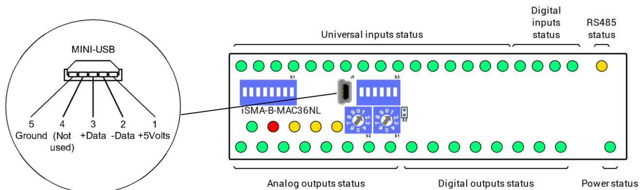
Figure 11. LEDs on the front panel of iSMA-B-MAC36NL.
