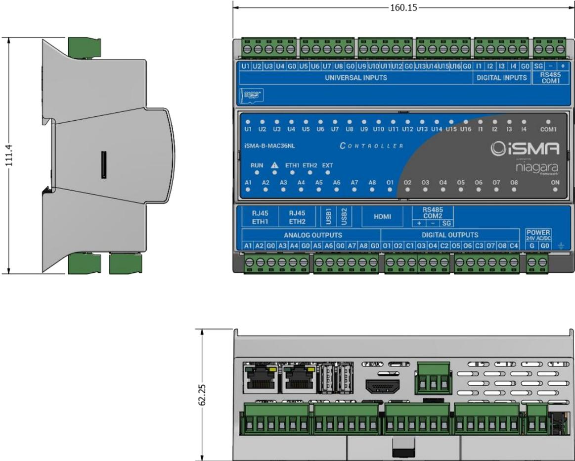
Figure 2. iSMA-B-MAC36NL Dimensions [mm]
