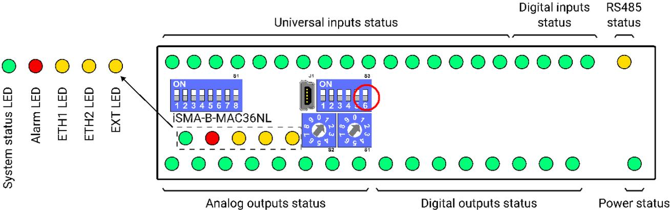
Figure 32. DIP switch view
