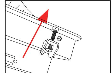
16.Then turn the long screw clockwise onto the snap plate to fix the machine. Generally, the two snap screws on the left and right sides
