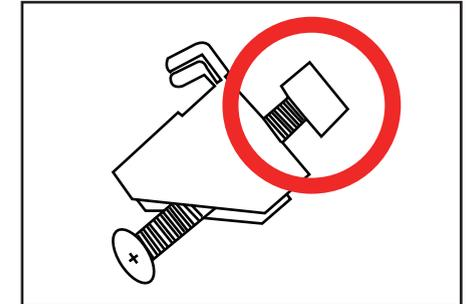
14.Lock the snap nut to the long screw, just lock it flat, do not bulge
