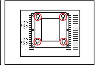
3.Use four fixing screws to align the fixing slot of the wall bracket and insert it. Gently move it to the under and insert to the fixing card slot.
