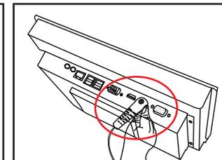
11.Plug in the power cord and plug in the power, presstart the machine with the silver machine start switch.
