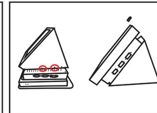
8.Place the triangle base in the aligned position, then fix it with M3 screws from both sides, finallypower on the machine.
