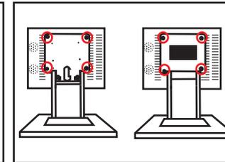
5.Fix the folding bracket to the machine with M4 screws, cover the decorative plastic cover, then twist it with the M3 screw
