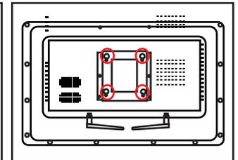
9. K-typed stand :First fix the fixing screws to the back of the machine to reserve space for the card to the bottom, then take out the base from the package and lay it flat.
