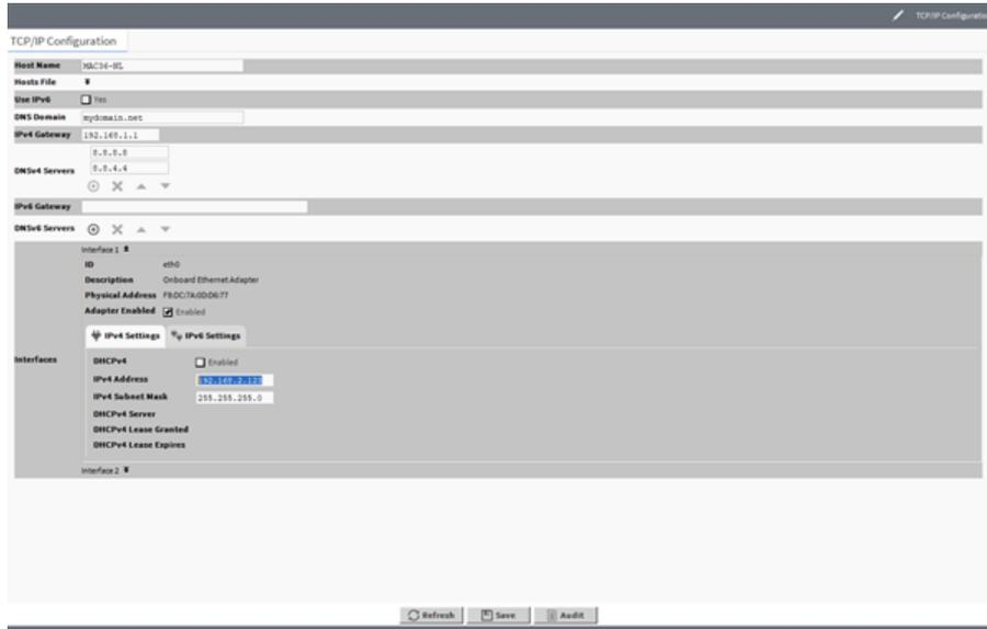
Figure 21. TCP/IP configuration
